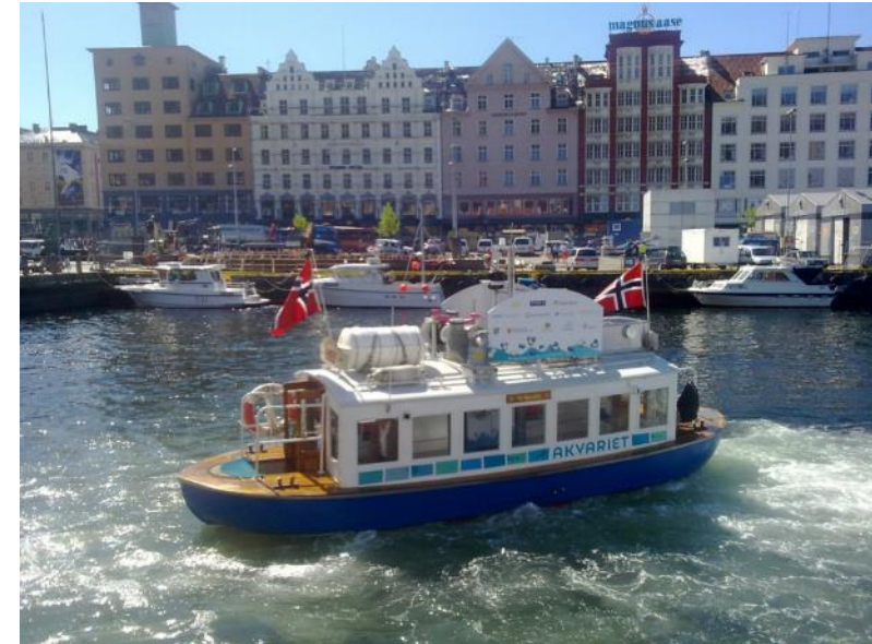
12,5 kW FC system inkl batteries and electric propulsion installed and tested on MF Vågen
