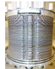
Light-weight FC and ELY stacks for Space Applications
