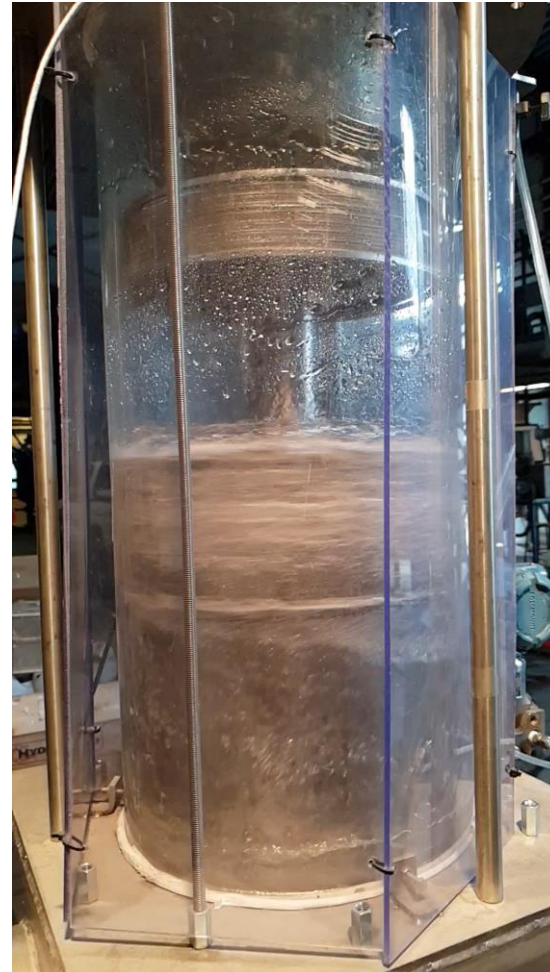
The patented RPB absorber lab test rig at USN/SINTEF testlab in Porsgrunn, Norway
