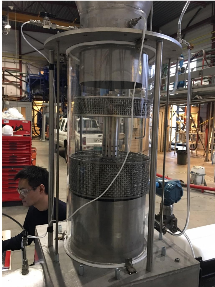
The patented RPB absorber lab test rig at USN/SINTEF testlab in Porsgrunn, Norway
